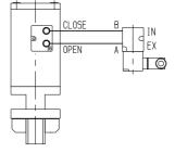
Compressed air pressure (min. - max. overpressure): 4 - 7 bar / 55 - 100 psig Use only clean, dry or slightly oiled air!
