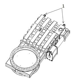
1 Load rings for valve lifting
