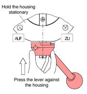
... and tighten the head cap screw to a torque of 9 Nm.
