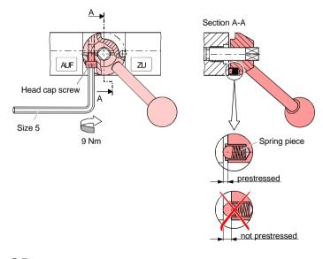
In this position, the spring piece for positioning the lever is prestressed.
