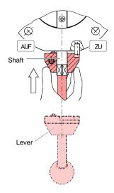
... and turn it counter-clockwise up to the stop position (pin).
