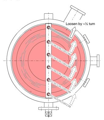
Tighten the hex socket cap screws with a torque of 11.5 ... 12 Nm.
