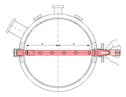
$\ldots$  and remove excess lubricant from the sealing surface.
