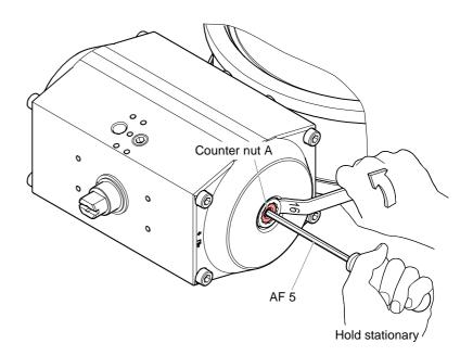
... and loosen adjusting screw A by 3 ... 4 turns.
