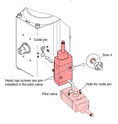
Establishing the compressed air connection
