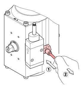
Connecting the compressed air outlets
