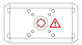
$\dots$  slide the actuator onto the square neck of the shaft and screw the actuator to the valve. Tighten the M8 hex socket cap screws with a torque of 20 Nm.
