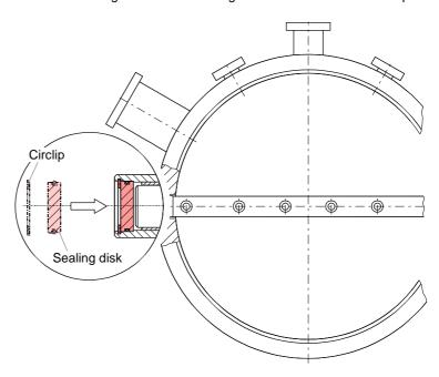
Mounting the O-ring to the valve plate
