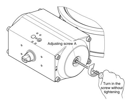
... and tighten counter nut A with a torque of 4.5 Nm.
