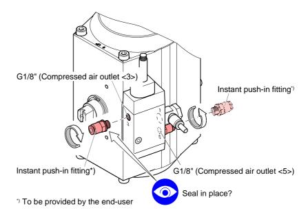
$\dots$  and mount the plastic tubes by pushing them into the instant push-in fittings until the mechanical stop is reached and check for correct mounting by slightly pulling.
