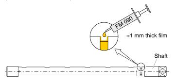
Slide the O-ring onto the shaft and insert it level into the groove without twisting it.
