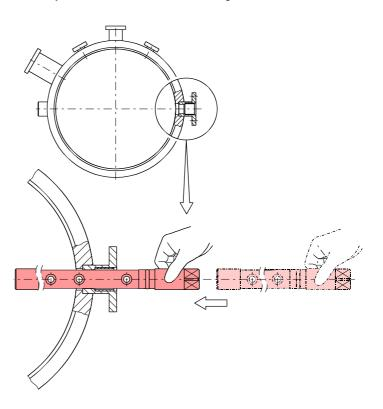
4 Lubricate the contact surfaces of the shaft and the visible surface of the O-ring by applying a thin, uniform FM 090 film.
