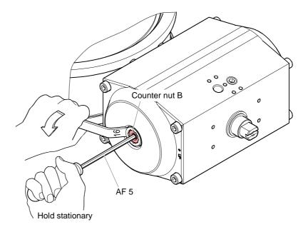
$\dots$  and turn in adjusting screw B by 3  $\dots$  4 turns.
