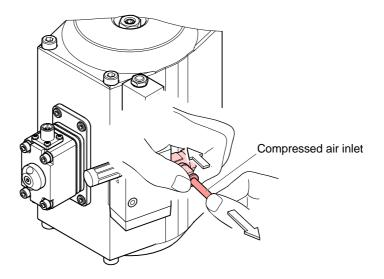
Press the rings of the compressed air outlets towards the valve and pull out the plastic tubes.
