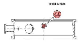
... and lubricate the sealing surface by applying a thin, uniform FU 090 film.
