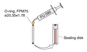
Install the sealing disk with the O-ring and lock them with the circlip.
