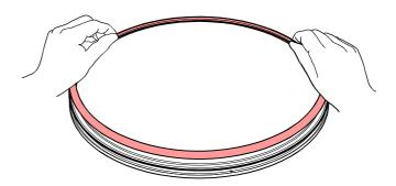
... and press it crosswise into the groove as shown in the illustration below.
