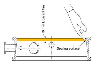
Pre-installing the valve plate
