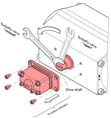
Power and compressed air failure
