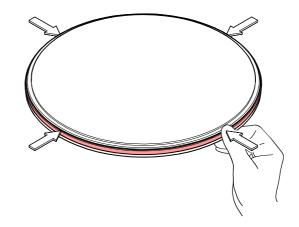
Press the remaining parts of the O-ring level into the groove without twisting the O-ring.
