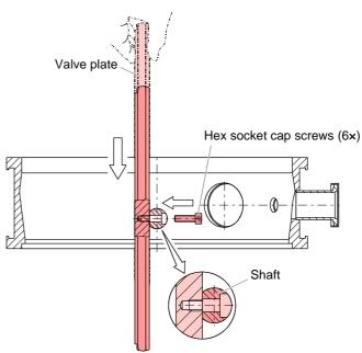
Tilt the valve plate by ≈45° and screw it to the shaft.
