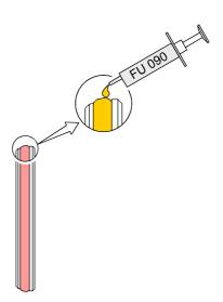
Lubricating the sealing surface
