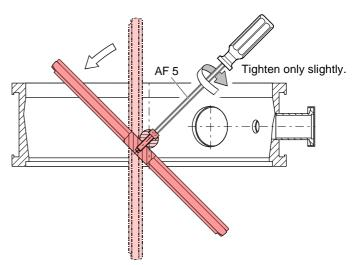
Centering and tightening the valve plate
