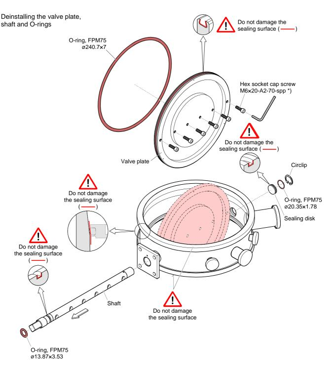
\*) The hex socket cap screws are secured with spp (stepstop®) and thus difficult to loosen.
