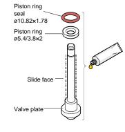
... and wipe the flange and valve plate seals with a lint-free cloth moistened with high vacuum oil (583413).
