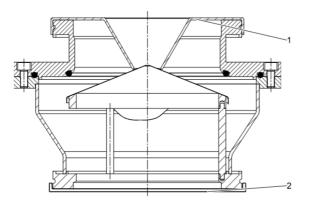
Illustration 5: Sectional view of valve transport fixation device
