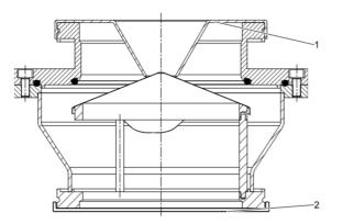
Illustration 2: Sectional view of valve transport fixation device
