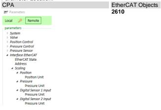
Note: The scalers for "Digital Sensor Inputs" are only visible if the sensor source is configured as 'digital'. See chapter «Sensor configuration».
