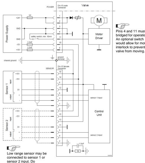
Pins 4 and 11 must be bridged for operation. An optional switch would allow for motor interlock to prevent
