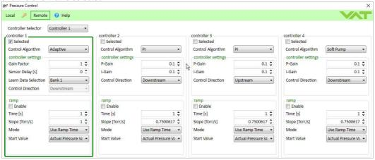
Alternatively, the **Automated Controller Selector** (see below) can select the controller depending on pressure ranges or control direction (up- / downwards).
