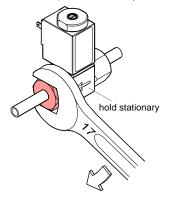
**7** Check that the vacuum connections are leak tight.
