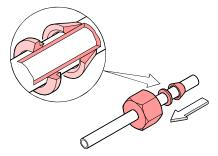
**3** Remove the protective lid and insert the tube until the mechanical stop is reached.
