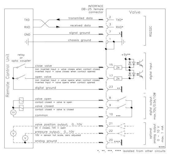
Do not connect other pins than indicated in the schematics above! Use only screws with 4-40UNC thread for fastening the DB-25 connector!
