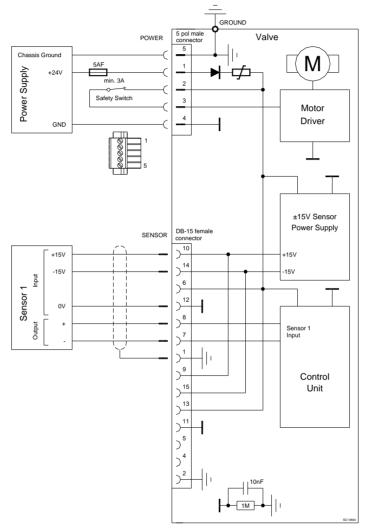
Pins 2 and 3 must be bridged for operation. An optional switch would allow for motor interlock to prevent valve from moving.
