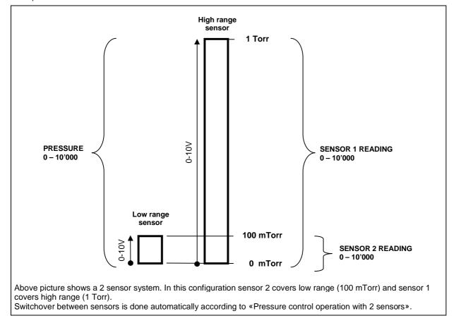
Example of PRESSURE and SENSOR READING allocation:
