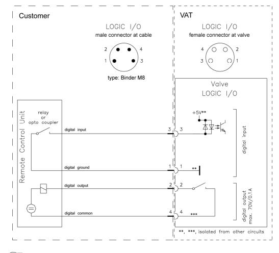
Do not connect other pins than indicated in the schematics above! Connector type: Binder M8 (99-3363-00-04).
