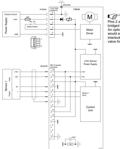
Pins 2 and 3 must be bridged for operation. An optional switch would allow for motor interlock to prevent valve from moving.
