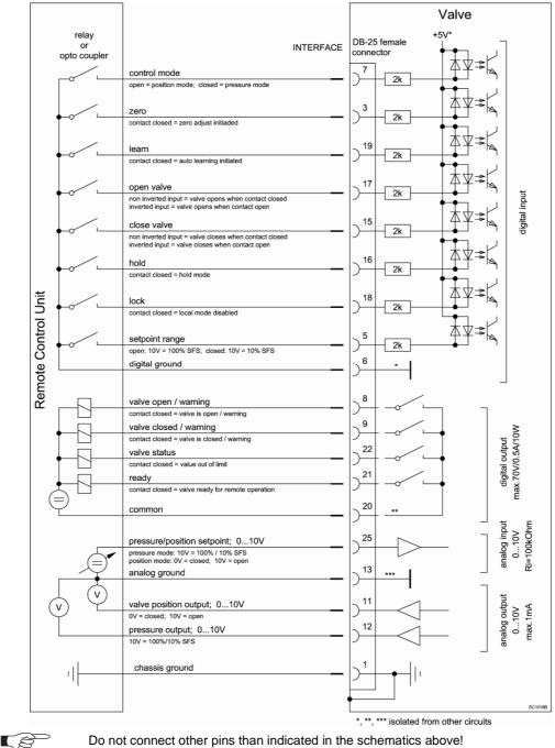
Use only screws with 4-40UNC thread for fastening the DB-25 connector!
