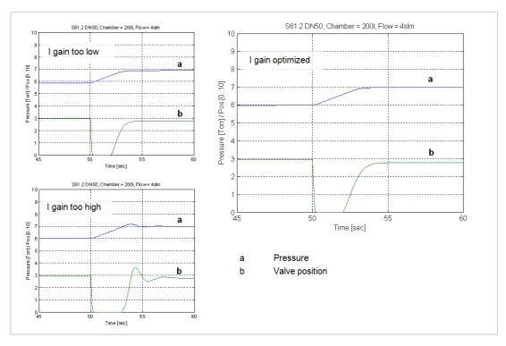
Check control performance over the whole control range with parameters above.
