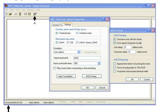
Acknowledgment that hyper terminal is connected to valve controller.
