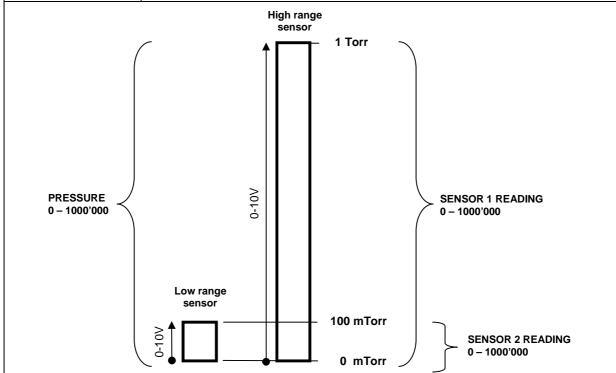
Above picture shows a 2 sensor system. In this configuration sensor 2 covers low range (100 mTorr) and sensor 1 covers high range (1 Torr). RANGE CONFIGURATION for PRESSURE resp. SENSOR READING is set to 1000'000. Switchover between sensors is done automatically.
