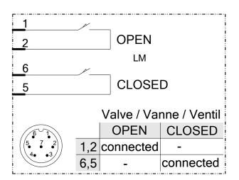
① LM Electrical connection for position indicator
