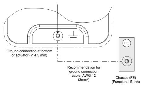
The connection point at chassis (FE) must be blank metal (not coated). It is also possible to connect the ground strap at system chamber if it is well connected to FE.
