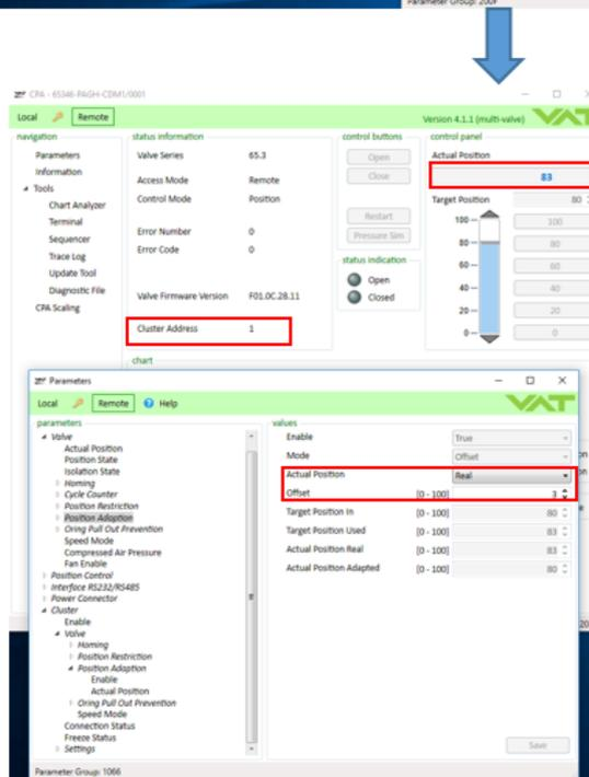
Picture : Position Offset with Actual Position - Real setting
