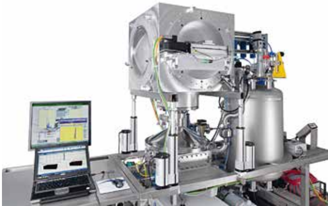
VAT particle test stand for particles > 10 nm
